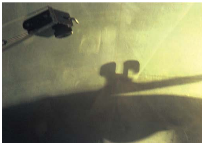
Fig. 4: Image of the bracket as seen on the screen of Starrett profile projector
